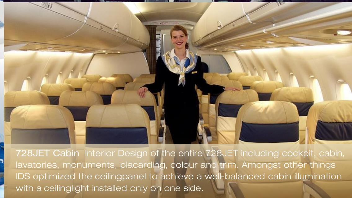
728JET Cabin Interior Design of the entire 728JET including cockpit, cabin, lavatories, monuments, placarding, colour and trim. Amongst other things IDS optimized the ceilingpanel to achieve a well-balanced cabin illumination with a ceilinglight installed only on one side.
