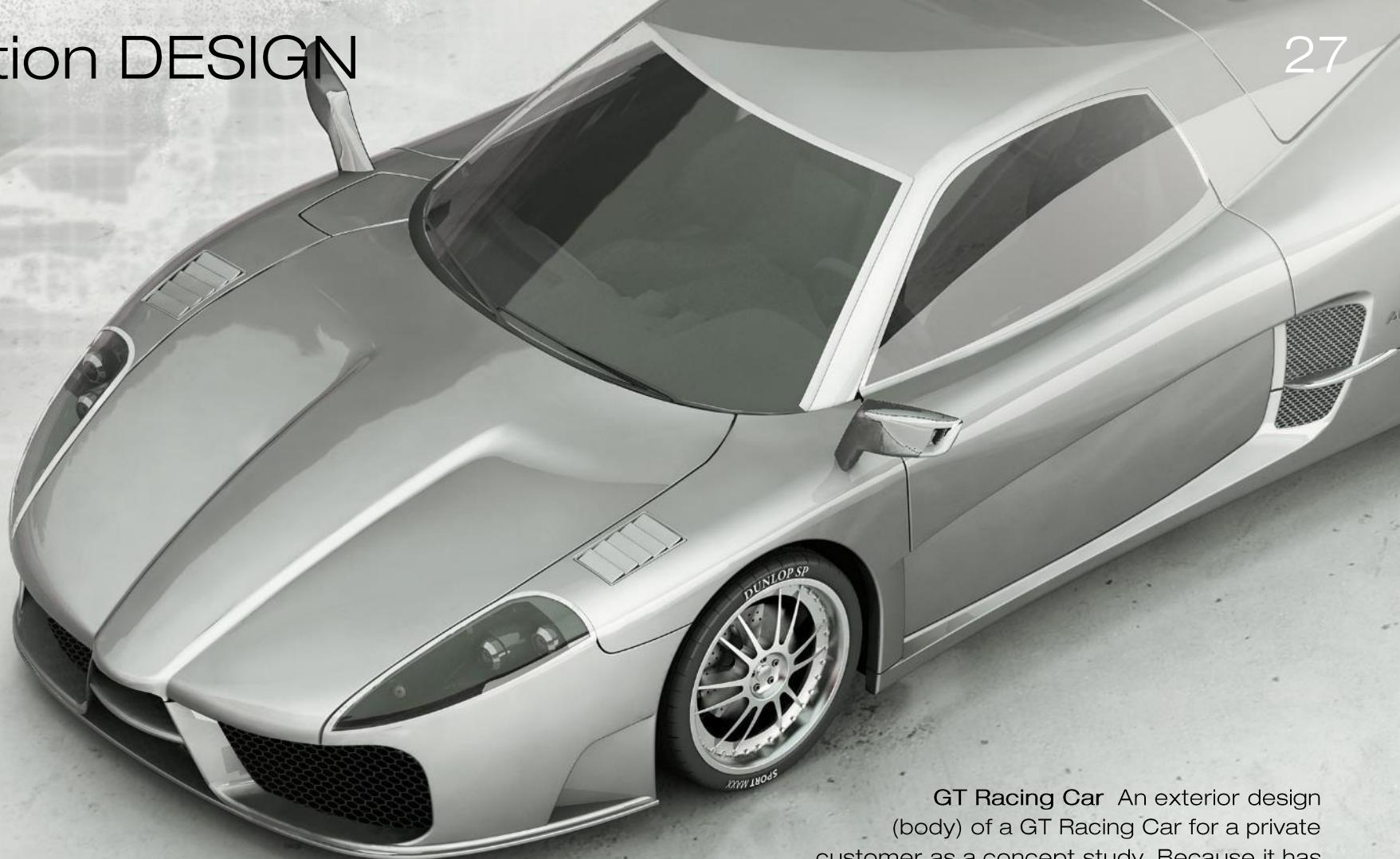
GT Racing Car An exterior design (body) of a GT Racing Car for a private customer as a concept study. Because it has been an individual development, it all had to begin with the analysis of the ergonomic dimensioning which led to a common package and finally to the construction of the car body surface data.
