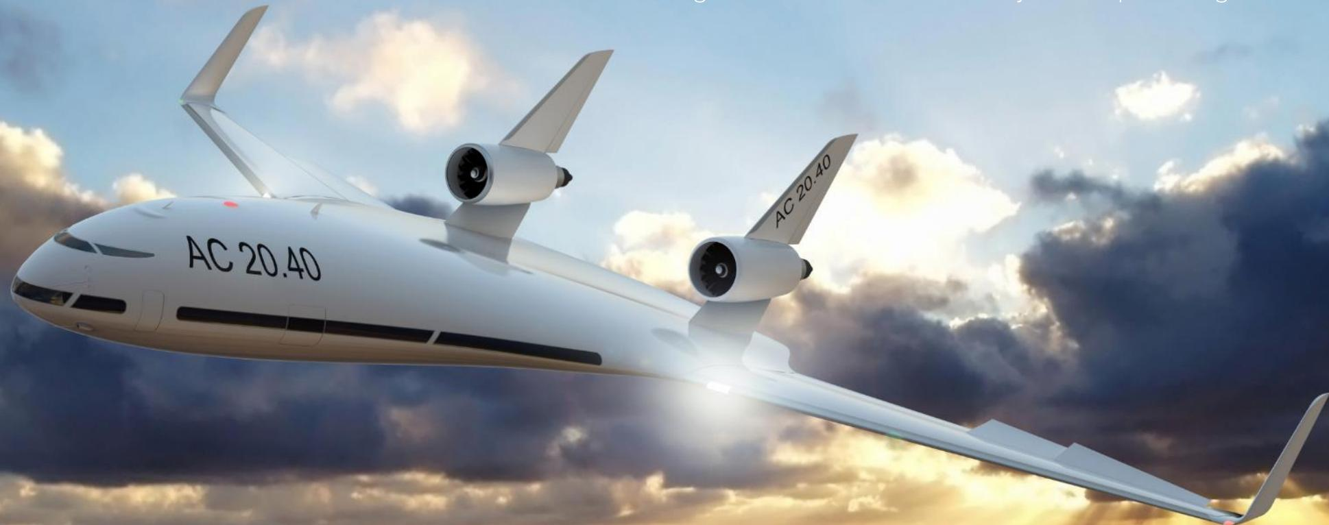
**AC20.40 Cabin Design** The project is supported by iDS with layout concepts, ergonomic research, graphic design/exterior and visualization. An airworthy model has already been developed by Prof. Werner Granzeier, HAW Professors and their students (Scale 1:30, Wing Span 2,70m). Various exterior, interior and research projects are in progress.
